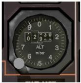
Figure 41: Standby altimeter
