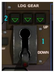
Figure 60: Landing gear control panel
