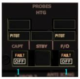
Figure 59: Probe heat panel
