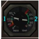
Figure 71: Oil indicator 1. OIL PRESS indication Green sector: 55-65 PSI Amber sector: 40-55 PSI Red mark: 40 PSI 2. OIL TEMP indication Green sector: 45-125 °C Amber sector: 125-140 C and below 0 °C  $\$  Red mark: 140 °C
