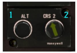
Figure 20: ALT / CRS 2 Panel
