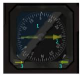
Figure 44: Radio magnetic indicator
