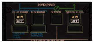
Figure 54: Hydraulic power panel
