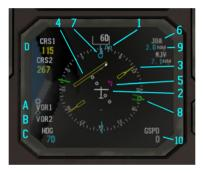
Figure 47: Electronic Horizontal situation indicator
