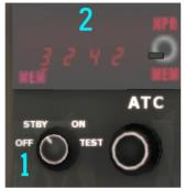
Figure 24: ATC control box
