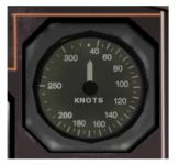
Figure 39: Standby airspeed indicator
