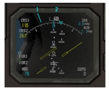
Figure 48: Electronic Horizontal situation indicator – arc mode
