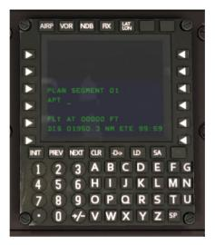
Figure 66: Modified FMC installed in the ATR 72-500
