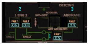
Figure 56: Engine / wing de-icing panel
