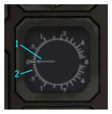
Figure 42: Vertical speed indicator
